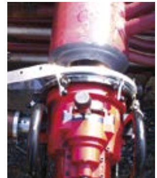
EP 424 SpeedPrep™ deluxe prepping heavy wall pipe
