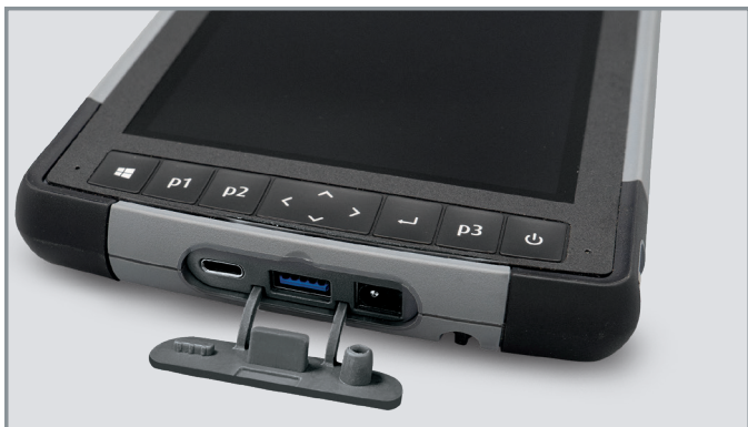
TC-110 power connection plus USB-A and USB-C slots.
